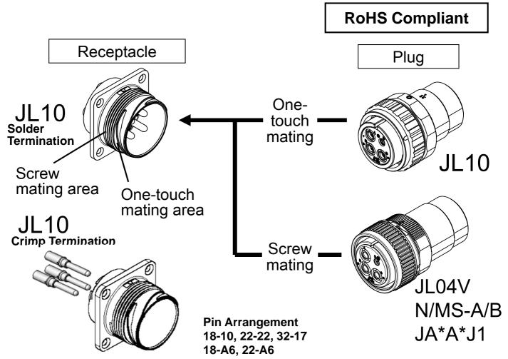
The JL10 Series are TUV approved and UL recognized, one-touch locking, circular, waterproof connectors for industrial machinery, satisfying European safety standards. The adopted Bayonet-style one-touch lock mechanism has a superior mating and unmating operability and the product contributes to an easy mating function.
