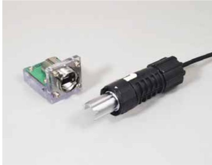
FO-BD7D is an optical pluggable connector for outdoor use which can be assembled on-site. This connector series addresses common thermal issues caused by optical modules by embedding the optical module into the FO-BD7D plug.
